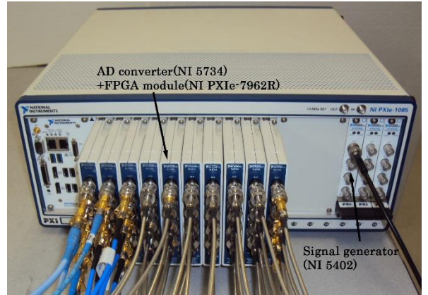
Fig. 4 Photograph of the PCI eXtensions for Instrumentation (PXI) system. 40 AD converters (NI 5734), FPGA modules (NI PXIe-7962R) and signal generator (PXI-5402) were set in the chassis.
