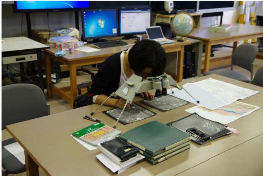
Figure 2.18 Picture of aerial photo interpretation (Miyagi, 2013) (performed using aerial photograph, stereoscope for aerial photography (mirror type), simple stereoscope, topography map, geological map, writing materials, etc.) The series of aerial photographs should be arranged as shown above, and be examined from directly above. The gap separating photographs differs depending on the person; fine tune the image by moving the photographs slightly until the image is clearly visible (Miyagi, 2013)
